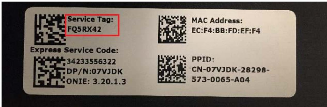
Figure - 2: Service Tag Location on the Device
